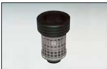
Protective valve. For safe lifts using fixed hooks/tools. Fitted between the lift tube and the vacuum box. Immediately eliminates the depression inside the lift tube if the load is released inadvertently.
